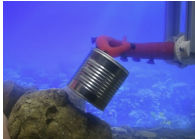
Developed by the Istituto Italiano di Tecnologia, the robotic arm integrates tactile sensors into its suction cups to grasp and manipulate objects autonomously, even underwater. Image: IIT
